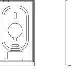
**DTV+ Digital Interface Mounting Bracket** 35/16" x 55/8" x 1" 84 x 143 x 25 mm
