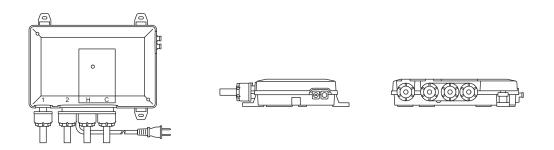
$\text{DTV}_{\tiny{\odot}}$  2-Port Digital Thermostatic Valve
